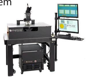
SA-12 semiautomatic probe system mounted on a vibration isolation table with an A-Zoom compound microscope and probe card holder - several configurations available.
